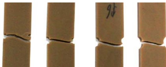
图5 切口试件断裂的宏观形貌 Fig. 5 Fracture topography of notched specimens
